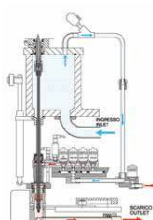
TANK GAS AND LEVELLING GAS CIRCUITS WASHING CYCLE
